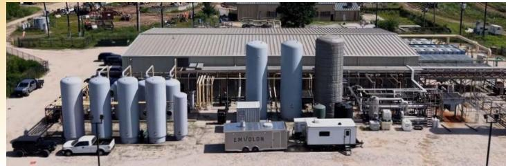
A Gold Prize is awarded to **Emvolon** in the **Advanced Renewable Fuels category** for presenting a technologically disruptive and globally scalable innovation. Emvolon's unique approach – repurposing automotive engines as chemical reactors for on-site methanol production from biogas streams – represents a clear break from conventional, highly centralised and capital-intensive e-fuel and e-methanol production pathways.
