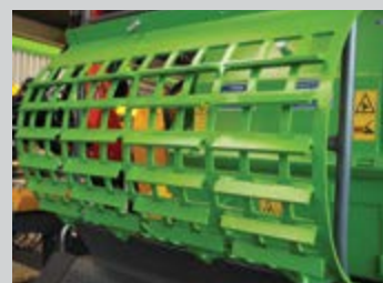
Grilles de calibrage : 25/25mm, 35/40mm 45/60mm, 60/80mm
